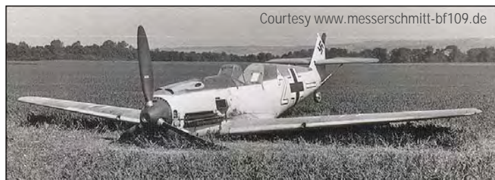
Bf 109 E-1 white 2 + - note the light grey (?) wing leading edge and gun throughs.
